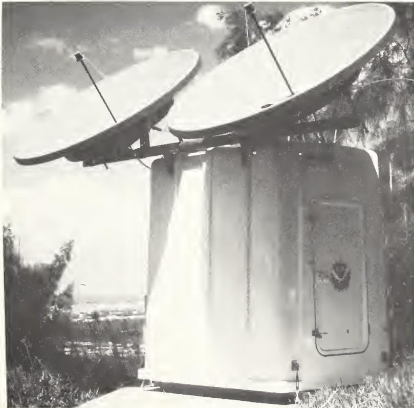
Figure 2-2.--TARS installation at Oahu, Hawaii. Note the rugged, self-contained design.
